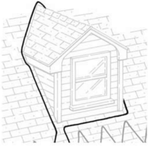
Figure 7. Cable pattern around a dormer
