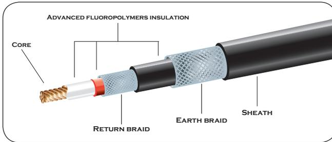
The product is designed for 240V supply installations- ensure the correct heater for the correct power supply has been purchased. Applications at 208V and 277V can be made effective with customized spacing of the heating cable. The cable produces between 10 to 20 Watts per sqft (100W to 200W/SQM) of heating, depending on the spacing of the cable (see Sizing Guide at the back of the manual). The product is CSA approved.
